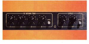
processors worked at roughly the same settings anyway, so there wasn't much need to tweak the levels. It was more important to set the processors' internal natch levels so that when switching between processors the levels still matched. This done. I set each processor to a different effect and balanced the quantity of each effect coming into the Ouad-FX with the four trim pots.
