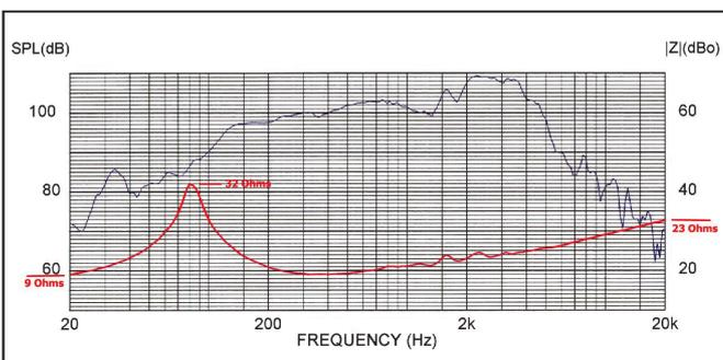
The red plot shows the speaker's impedance curve and proves that it varies according to the frequency of the signal being applied to its terminals.
