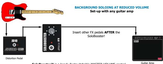
**SoloBooster™** is a handy footswitchable MASTER VOLUME control that can be used to lower the volume of your soloing sound for use behind a vocal. Then when it's time for your solo you just step on the footswitch for full-on solo volume - easy
