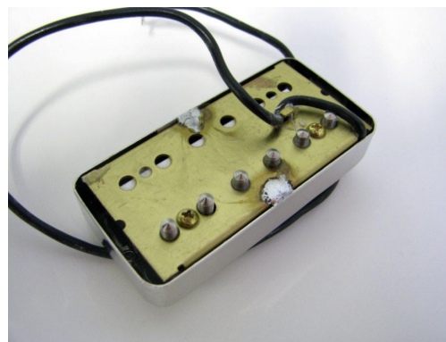
Left - The excellent Gretsch style 'HiLoTron' pickup from TV Jones on a black Gibson mount. Right - An underside view showing similarity with the P90
