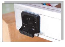
blowing when you switch on your amplifier. It is not possible to switch between AC voltages. The AC voltage is pre-set at the factory.
