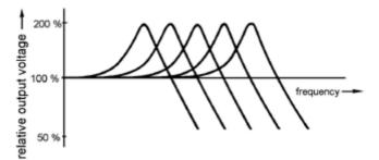
What's causing extra top end output? - All guitar pickups have a strong peak of output at frequencies which can range from 2000Hz to 6000Hz. The actual peak frequency can be raised or lowered by the capacitance in the guitar's wiring circuitry. The guitar cable's capacitance will also change the peaks. As shown by the
